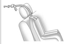
If the position you are using has a fixed headrest or head restraint and you are using a single tether, route the tether over the headrest or head restraint
